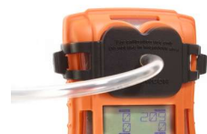
Bump/calibration plate To apply test gas to T4
